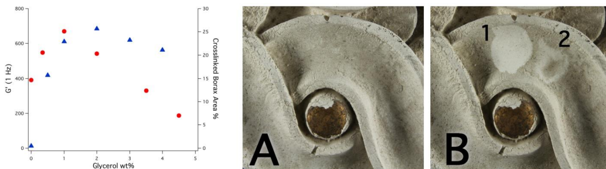
Figure 1: On the left, Storage modulus values at Frequency=1Hz (■) and Crosslinked Borate Area obtained from NMR measurements (▲) are plotted against glycerol concentration. Pictures on the right show the stucco surface before (A) and after (B) the cleaning, with the comparison between the the HPG based system (1) and a wet cotton swab (2).
